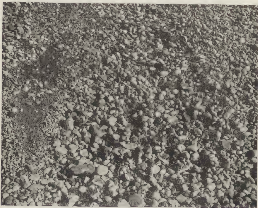
FIG. 10.—In some parts of the gravel bank the material consists almost entirely of coarse particles.
